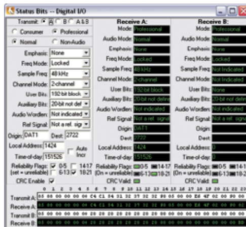
Complete Status Bit metadata setting and display for either consumer or professional format.
